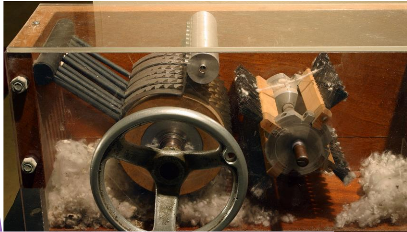
The cotton gin invented by Eli Whitney
